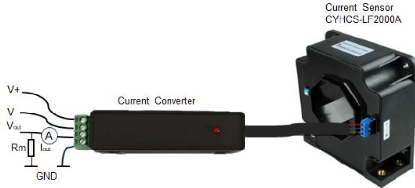
Fig.3 Connection between converter and sensor
