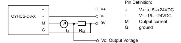
Measuring resistance  $R_M = 10\Omega \sim 100\Omega$
